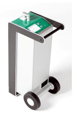
filter. The alpha and beta decays on the filter are measured by a high-end semiconductor radiation detector (1200mm²). This allows a perfect separation of the different decay products. The spectrometric analysis allows e.g. the detection of Plutonium aerosols which cannot be detected by measuring gamma radiation.
