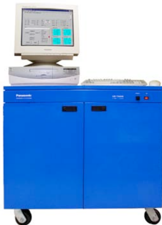
Figure 12 – UD-7900M Automatic TLD Reader.
